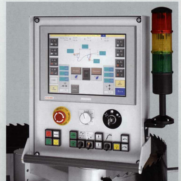
Well-arranged programming and operation of the machine by touch-screen. Programmes can be changed during working process.
